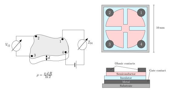
Left: Schematic of Van der Pauw's method for measuring the conductivity. Right: Layout of a semiconductor device for characterization.
